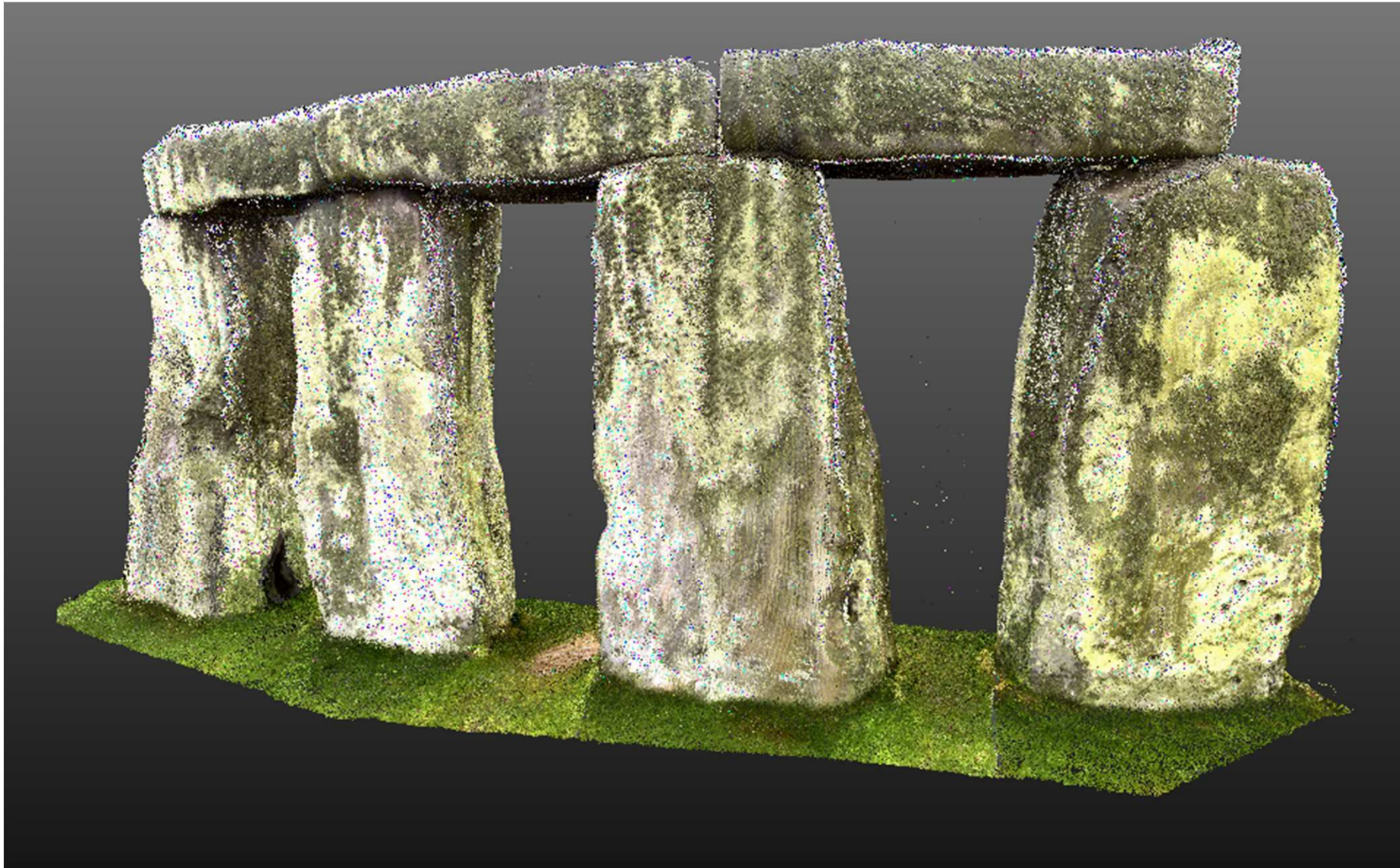
Example of a selection of stones in coloured point cloud form, prepared for initial mesh modelling.
