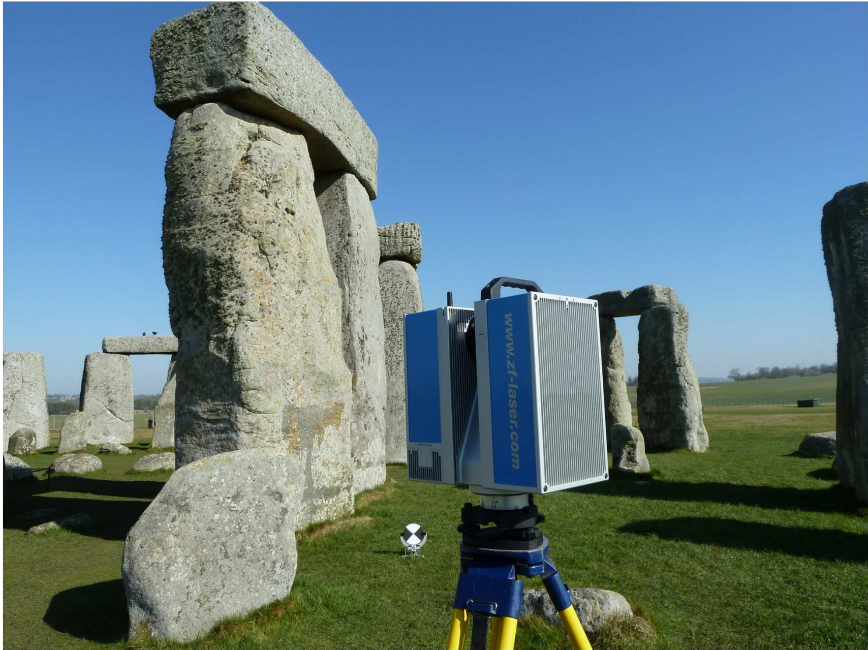
Use of the Z+F imager 5010, high resolution laser scanner within the stone circle.
