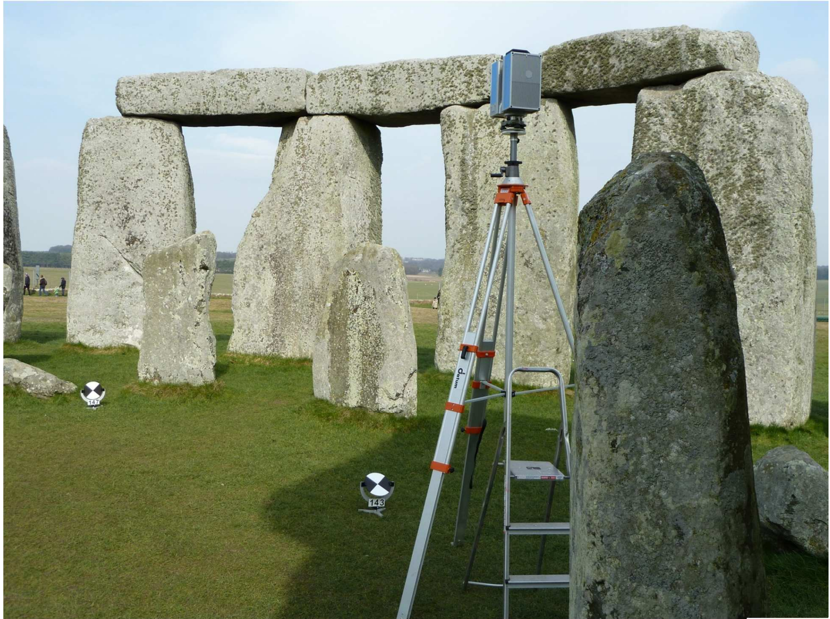
Example of high level laser scan coverage to the stone circle using an extendable tripod.
